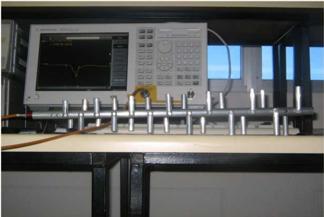
Figure 5.6 LPDA under bandwidth test
